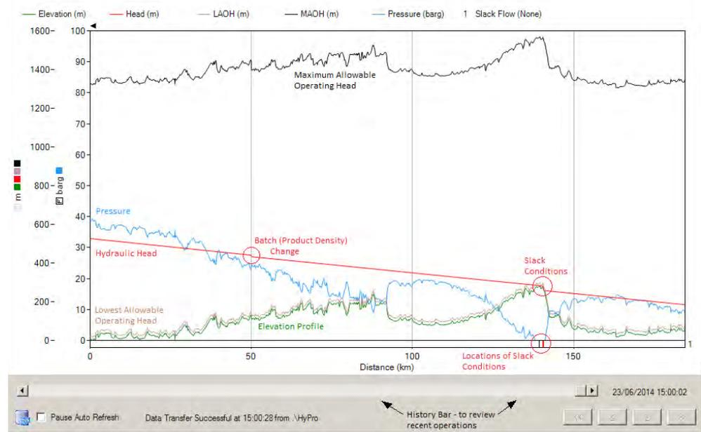
Atmos Hydraulic Profiler showing slack conditions at the 140.5 km mark
