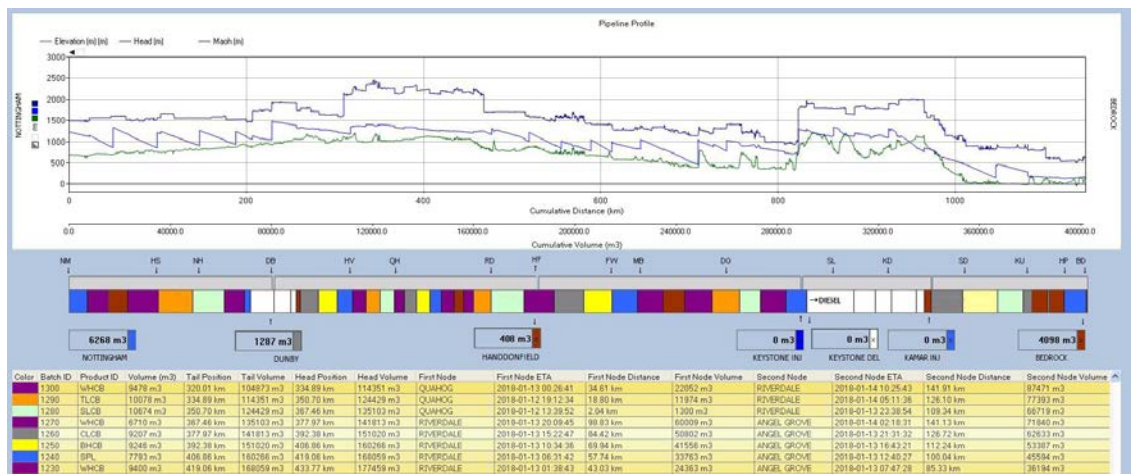
Hydraulic profile, and graphical and tabular, display for batches in a long pipeline with drastic elevation changes
