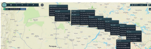
Figure 3. An example in Brazil of proposed flow and pressure set points recommended by simulation tools.
